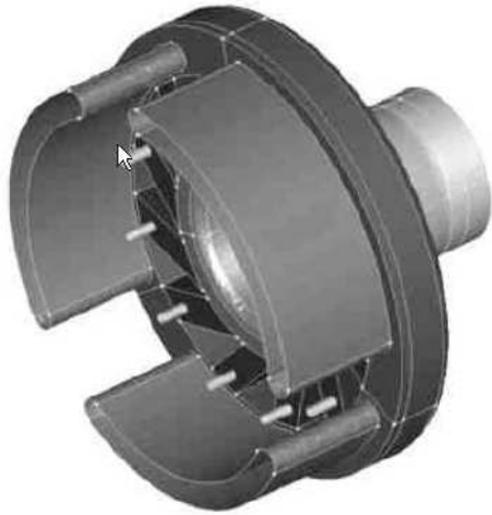
Figure 7.3: Backside view of the swirler with the three air inlets and twelve fuel injectors [177]
