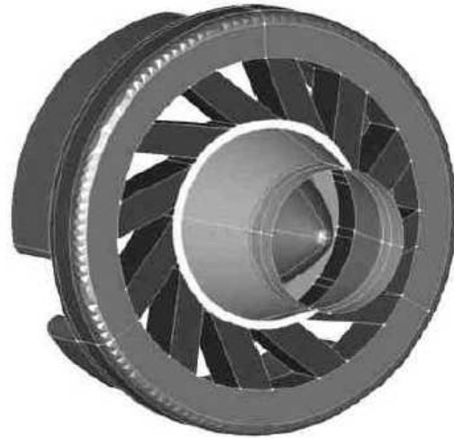
Figure 7.4: Front side view of the swirler and detail of the twelve arms which gathers in one exit [177]
