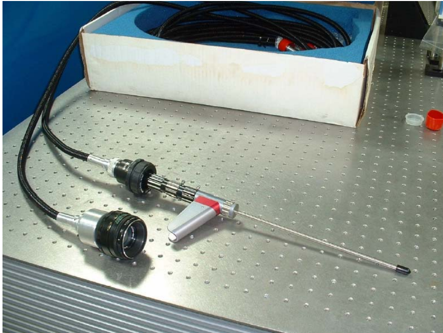
Figure 8.2 Photograph showing fibre bundles coupled to an SLR camera lens and a boroscope.
