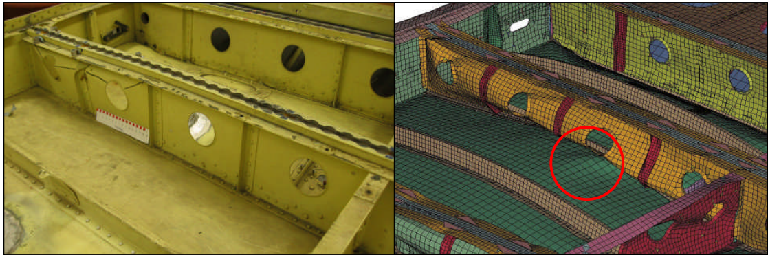
Figure 10 Separation that occurs due to an instability that develops in the water component on the reverse side of V480P shown in this figure
