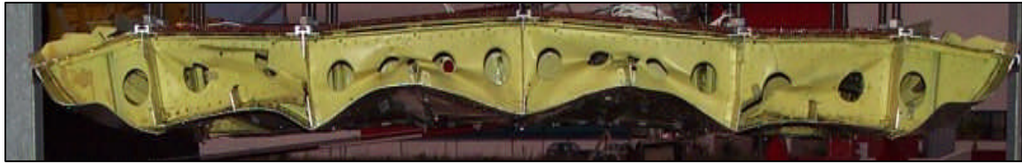
Figure 5 Deformation experienced along STN370A at the forward section of the sub floor
