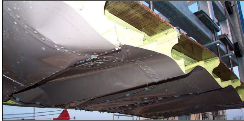
Figure 16 Underside view of the port side taken after the drop test. Picture courtesy of CIRA [11]
