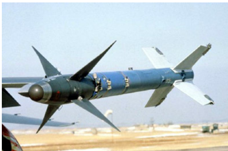
Figure 3-8: AIM-9L a Second Generation Seeker System (source [FAS07])
