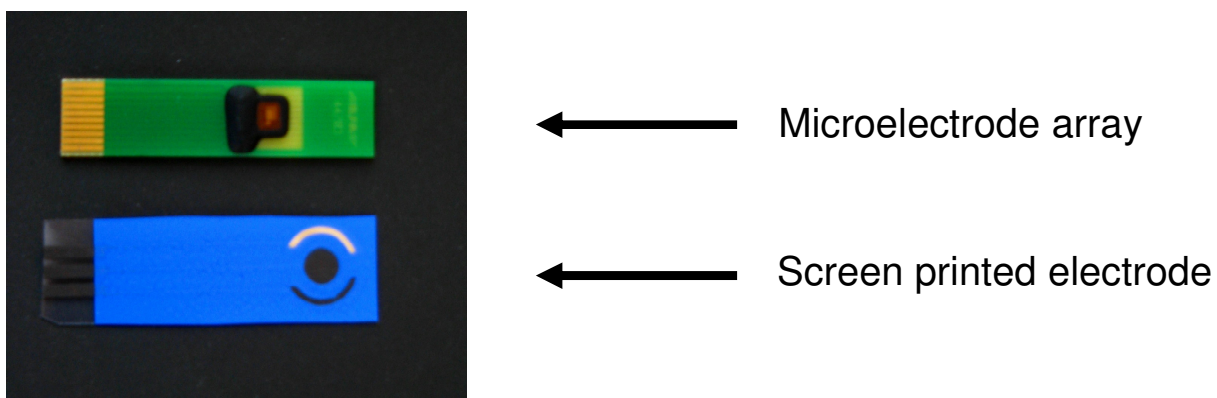
Figure 4.1: The microelectrode array from Tyndall National Institute and the in-house fabricated screen printed electrode.
