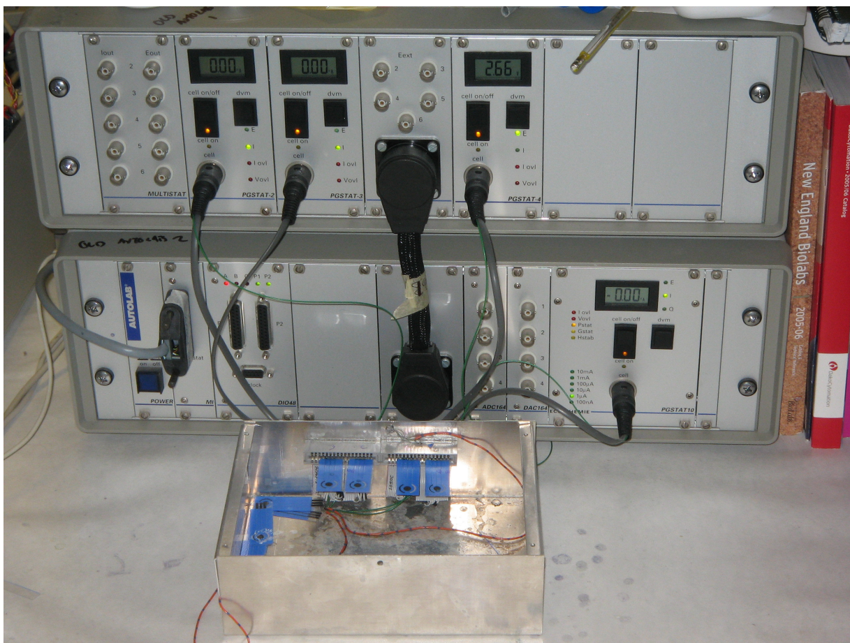
Figure 3.2: The Autolab instrumentation from Eco chemie used for the electrochemical measurement.
