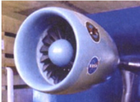
Figure 2-18: The advanced ducted propulsor fan. (Courtesy of NASA, P&W)
