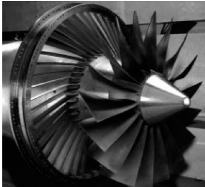
Figure 2-17: Leaned and swept stator vanes.
