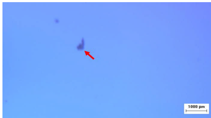
Figure 4.4 Magnetic resin bead agglomerate of 400 \mu\text{m} equivalent diameter.
