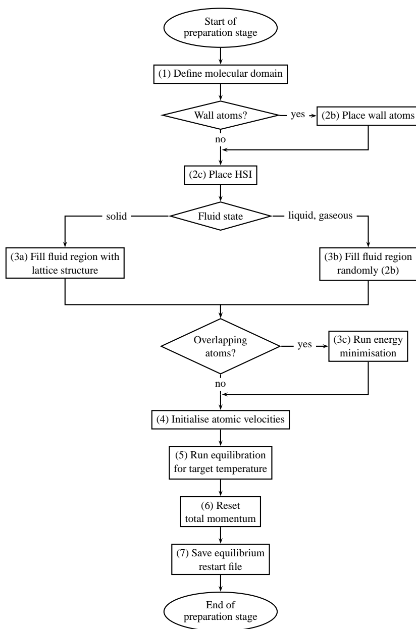
Figure 6.4: Flow chart of the preparation procedure to obtain the starting point for investigation of the MD flux boundary conditions schemes.
