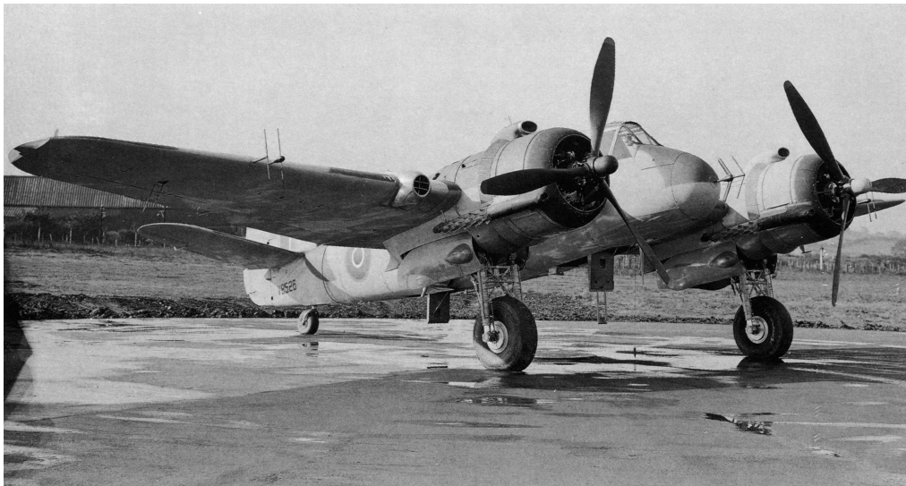
Fig. 96 Beaufighter with AI IV vertically-polarised aerials visible on the nose (transmitter) and wing (receiver). (Bristol Aeroplane Company /BAe).
