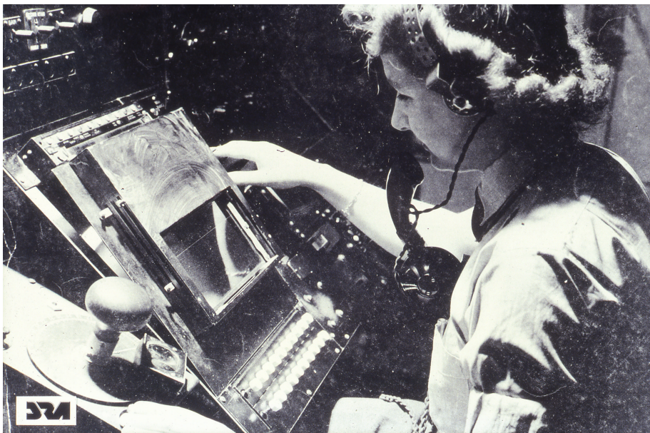
Fig 45. A WAAF Chain Home operator, Denise Miley. Her left hand is by the goniometer control and her right is ready to select direction- or height-finding. (IWM CH 15332).
