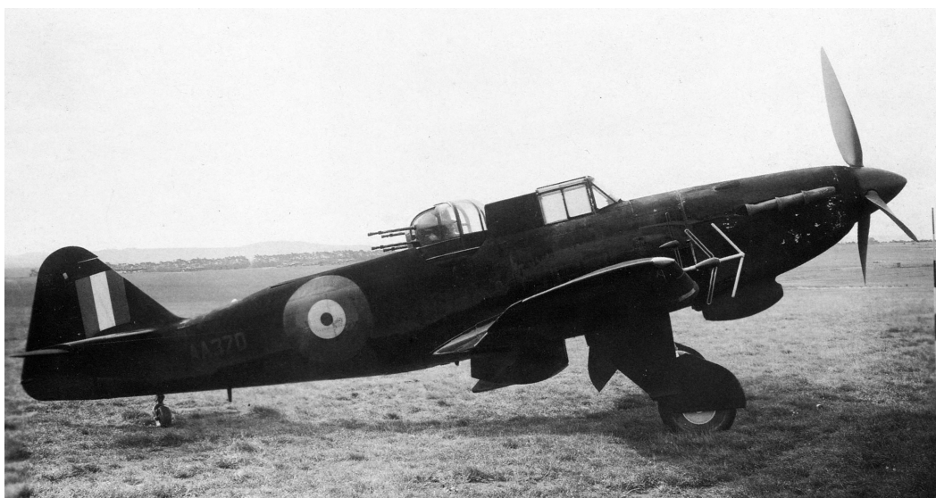
Fig. 97 Defiant fitted with AI IV – the transmitter aerial is visible on the nearer wing. (Phillip Jarrett /Robert Jackson, Air War at Night , Shrewsbury: AirLife, 2000, p.46).
