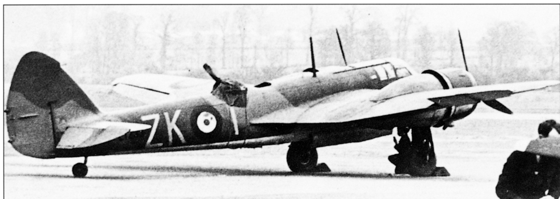
Fig. 84. 25 Squadron Blenheim in February 1940. The aircraft does not appear to have the underbelly gun-pack fitted as the bomb doors are open. (Jon Lake, Blenheim Squadrons of World War 2 , London: Osprey Publications, 1998, p. 62)
