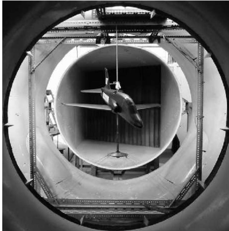
Figure 1: 4DoF rig with 1/12 scale BAe Hawk
