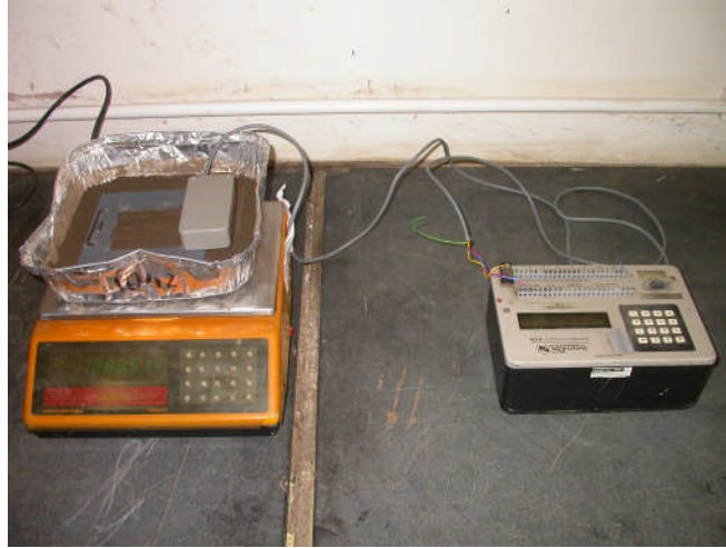
Figure 3.3 Calibration of soil moisture sensor using a Campbell data logger and balance.
