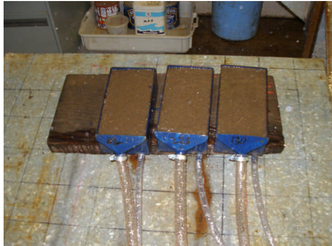
Figure 7.4 Microcosms under rainfall simulator. Run-off was collected by a funnel at the down-slope edge of the microcosm, and then directed through the larger gauge plastic pipes attached to the surface of the microcosms. Infiltration was collected from the thinner gauge plastic pipes at the base of each microcosm.
