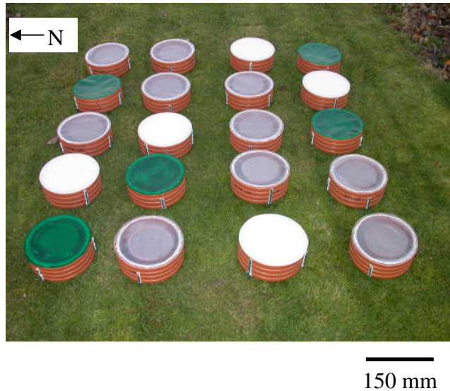
Figure 6.3. Microcosms and light filters in a randomised block design.
