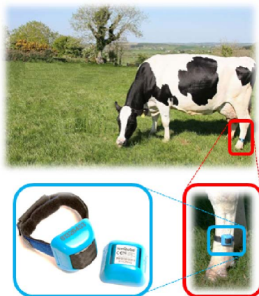
Fig. 2. IceQube sensor attached to the hind leg of a cow. Photos: Courtesy of IceRobotics Ltd.
