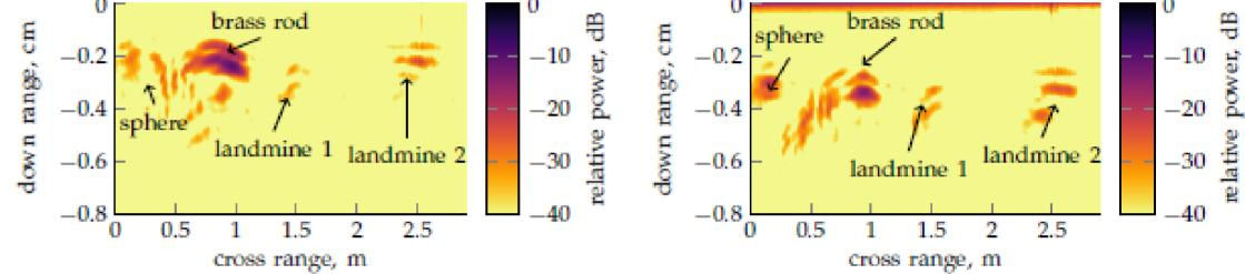
Fig. 3: Co- and cross-polar Yamaguchi polarimetric clutter suppression.
