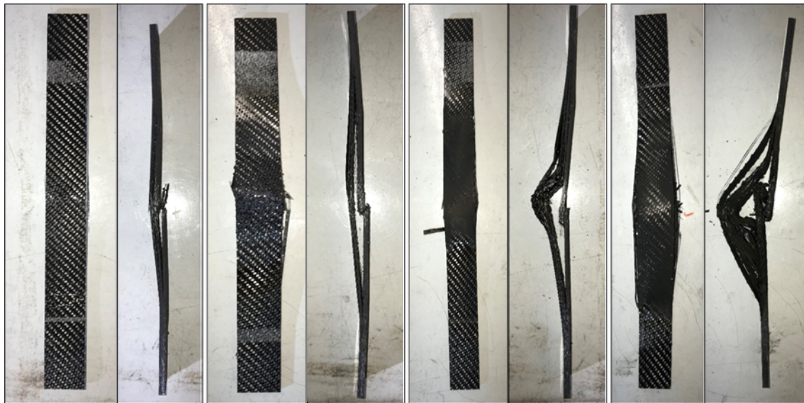
Figure 5 – Post-fire photograph of the bending samples showing left to right, 10, 20, 30 and 40 kW/m 2 .
