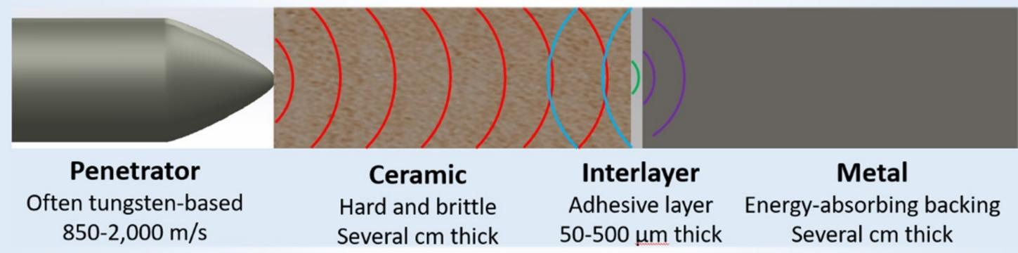
Controlling the passage of shock waves (generated upon impact) through this interlayer could potentially minimise damage to the ceramic, increasing erosion of the incoming projectile. This control would be achieved through optimisation of interlayer **acoustic impedance** - a property governing how acoustic waves (and shock waves) pass through materials.
