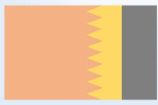
3D-printed ceramic with brazed metallic interlayer 100 µm thick High impedance Disruptive to shock wave
