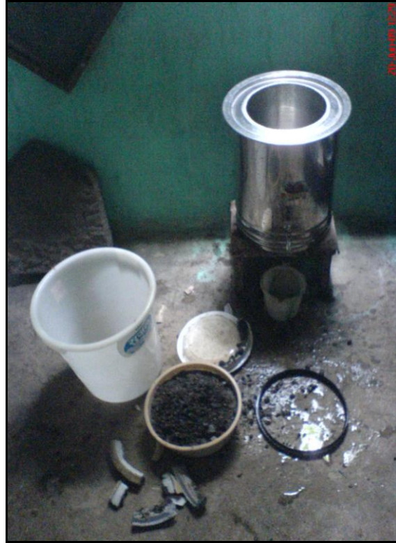
Plate 4: Broken bio-sand filter
