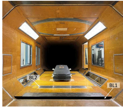
Figure 2: 8x6 Wind Tunnel at Cranfield University
