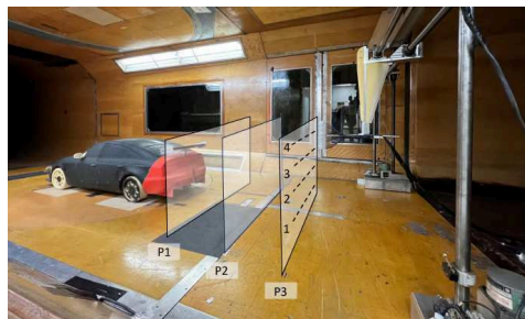
Figure 6: Wake total pressure measurements setup
