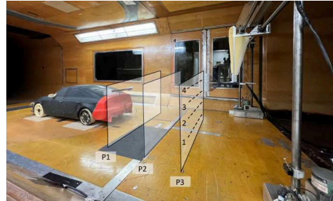
Figure 6: Wake total pressure measurements setup
