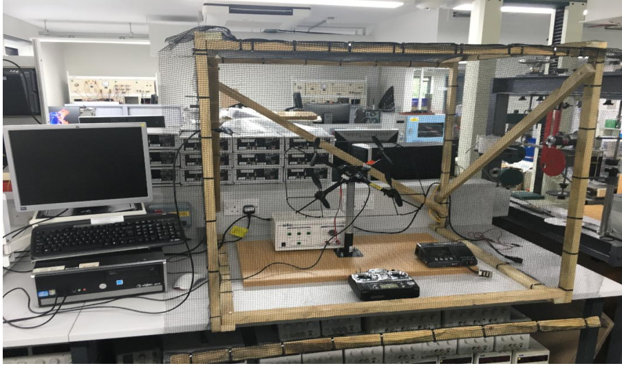
FIGURE 5.6: Quadrotor system with complete hardware test frame design for ILC controllers.
