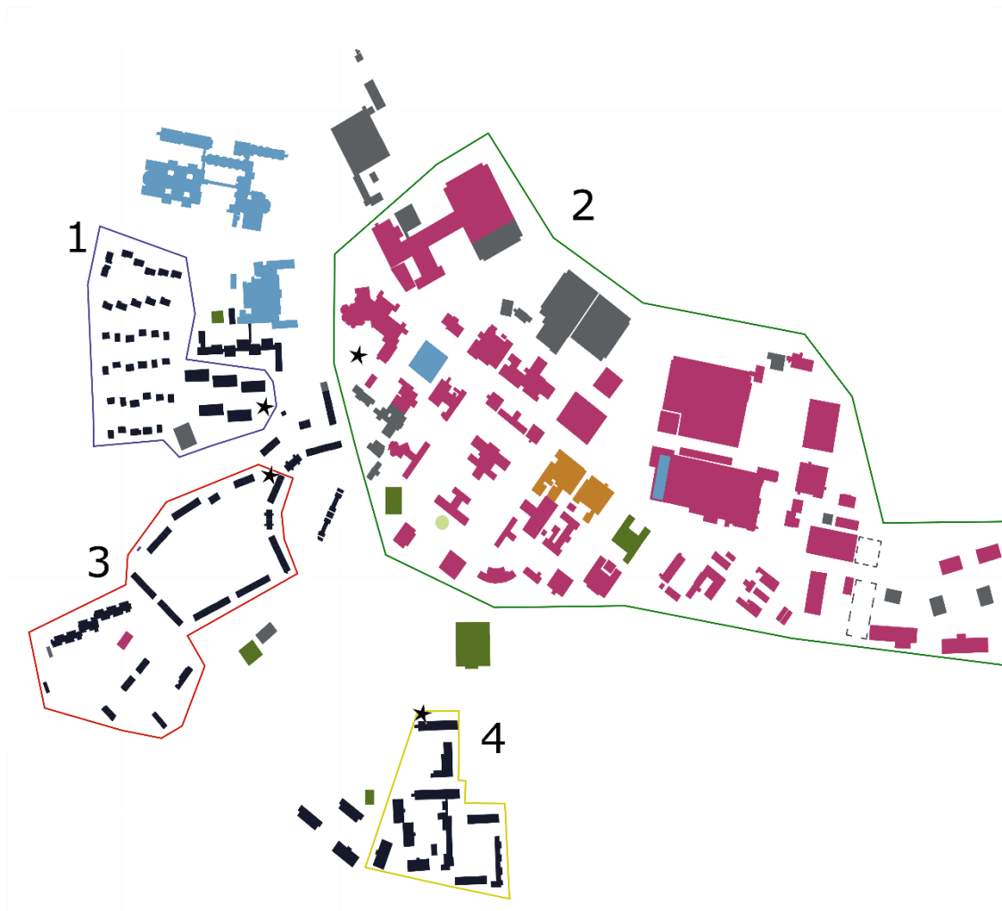
Figure 3: Cranfield Campus drainage areas which were sampled. 1- Halls of Residence A, 2 – University Technical Buildings In-Sewer, 3 – Residential Houses In-Sewer and 4 – Halls of Residence B. Stars indicate location of sampling point. Map not to scale.
