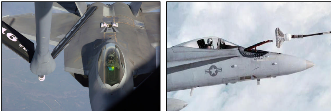
Figures 2 b and 3 c Illustrating boom refuelling and probe and drogue refuelling.
