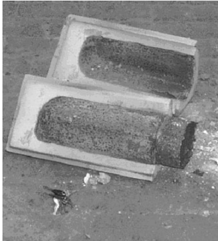
Figure 36 Typical vacuum induction melting furnace stainless steel ingot and crucible (United States Department of Energy, Albany Research Centre, Albany, Oregon)
