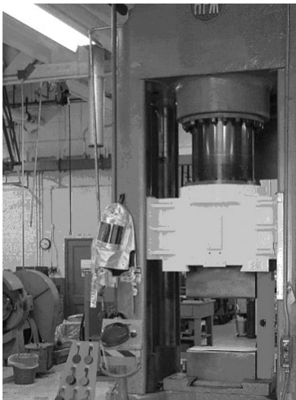
Figure 17 Forge used to upset cast austenitic stainless steel ingots (United States Department of Energy, Albany Research Center, Albany, Oregon)
