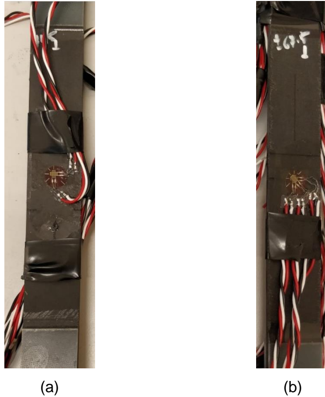
Figure 4.5 Position of (a) biaxial and (b) 45° rosette type strain gauges
