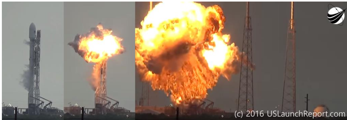
Figure 1.1 SpaceX Falcon 9 rocket explosion in Cape Canaveral due to helium storage CPV failure [6]
