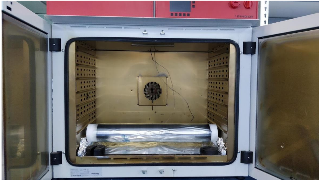
Figure 4.9 Pipe wrapped with shrink tape for curing in the oven
