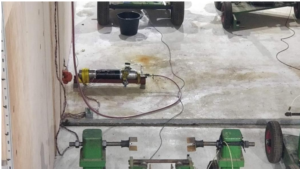
Figure 4.18 Pressure pit for pressure testing
