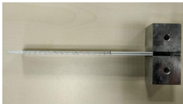
Figure 4.4 Mode I DCB specimen
