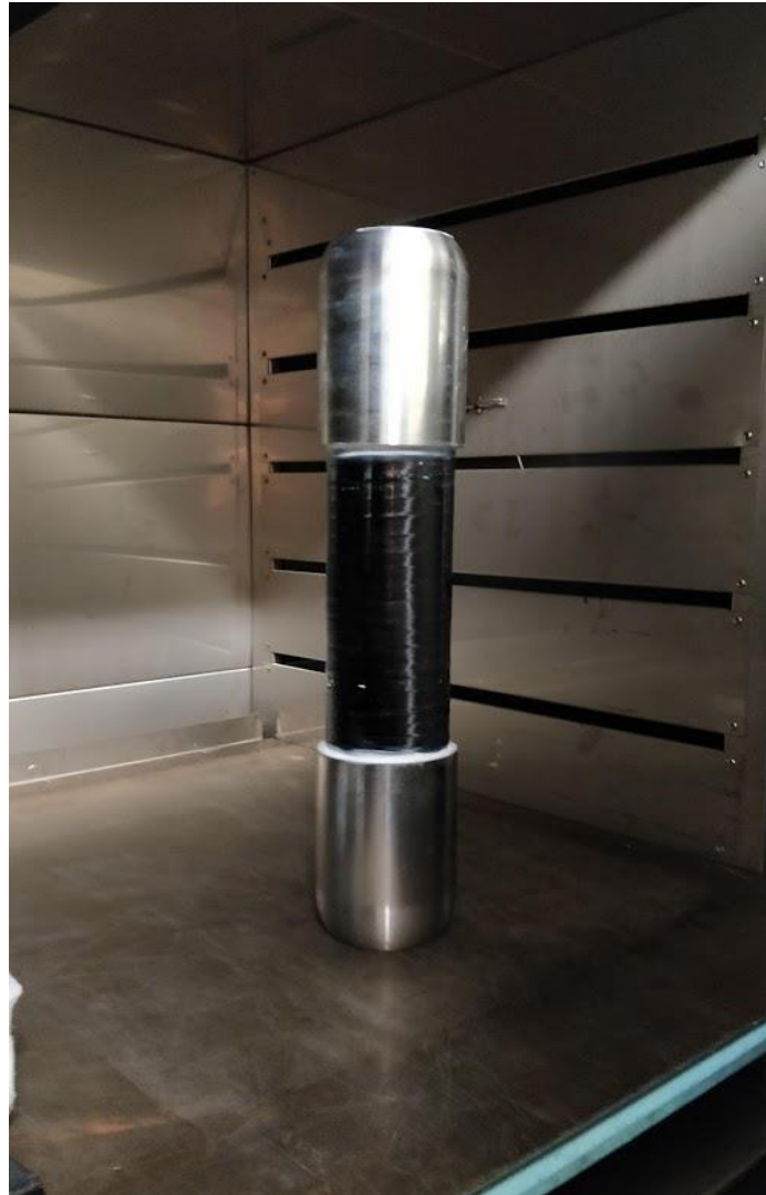
Figure 4.14 Adhesive bonding of end caps on pipe through curing
