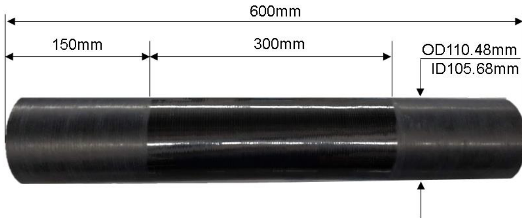
Figure 4.11 Treated areas of pipe for bonding
