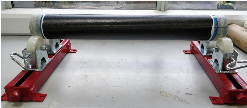
Figure 4.8 Set-up of composite pipe and bench top pipe rollers
