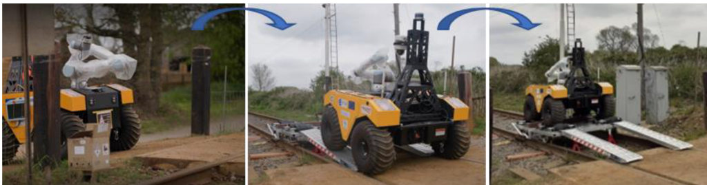
Fig. 17. Rail-road conversion at the footpath crossing at the NLR test-site.
