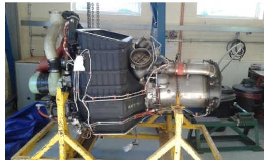
Figure 1-1 The Auxiliary Power Unit – a. Boeing 747-200 [5], b. The Boeing 747 APU that was used to set the test rig for this project installed on its cradle
