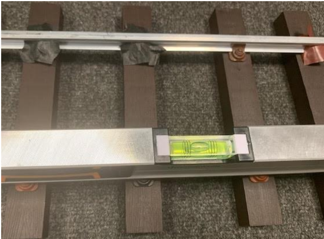
Figure 25: Leveling Measurement for the Track
