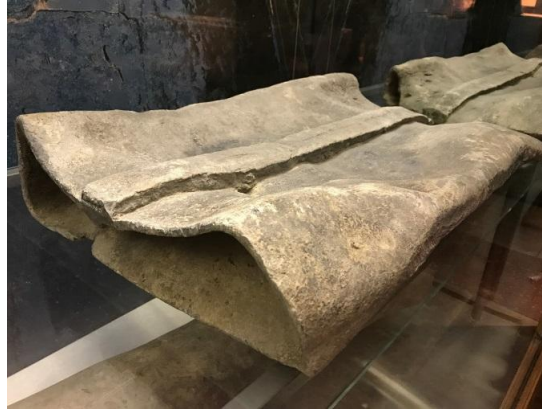
Figure 1.1: A roman water pipe made from sand cast lead sheet [6]
