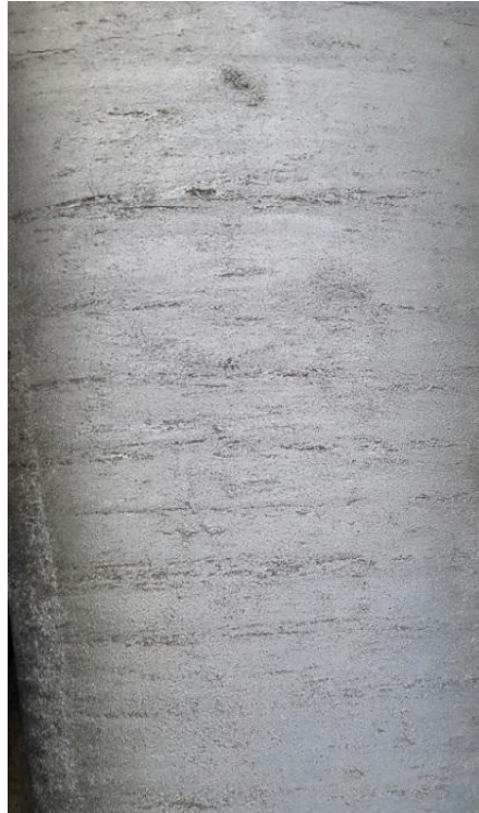
Figure 4.1: Sand side of cast sheet with grooves (60cmX100cm)
