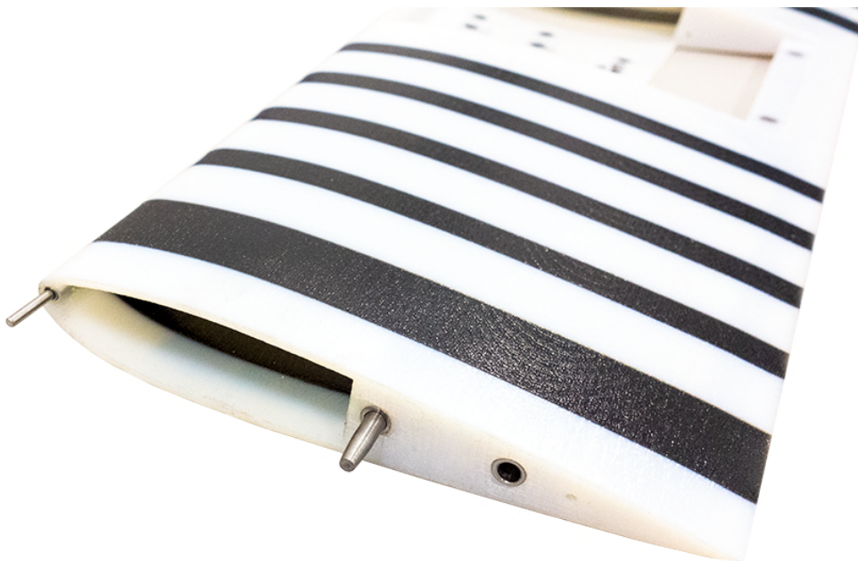
Fig. 6.18.: Section of the skin with the connection dowels and the flexible stripes well visible.
