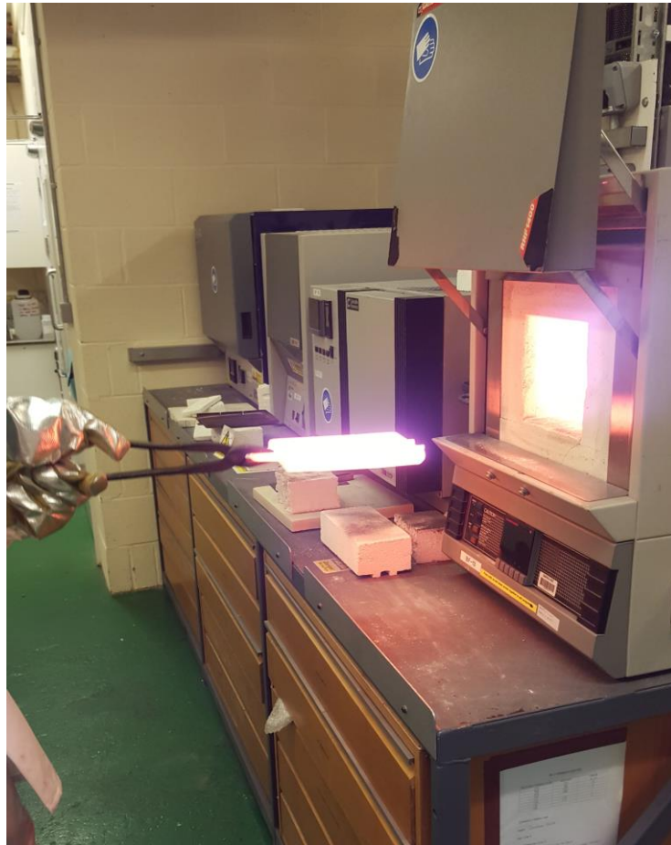
Figure 58 – Extraction of samples in-between oxidation cycles at t = 016 hours, before the sample is allowed to cool in their holder on a ceramic brick.
