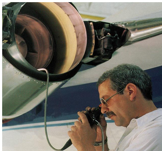
Figure 11 - application of visual inspection via borescope on an aero engine, courtesy of NDT Education Resource Center, Iowa State University, USA [51]
