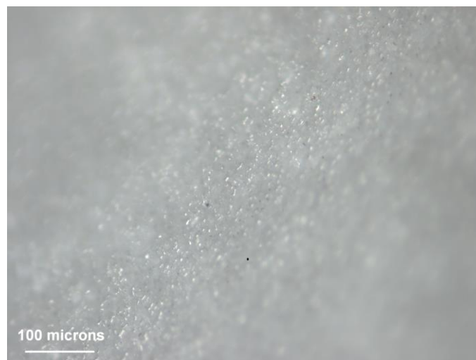
Figure 56 – Micrograph (10x zoom) of post-furnace sample S05 at t = 16 , showing the coating free from soot.
