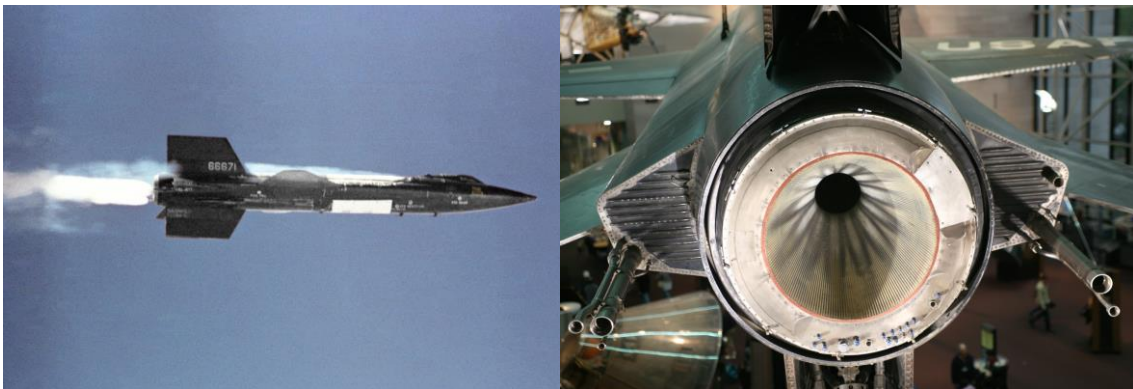
Figure 6 - NASA/USAF experimental research aircraft X-15 (left) [32], where TBCs saw one of their first applications in the rocket nozzle (right) [33]
