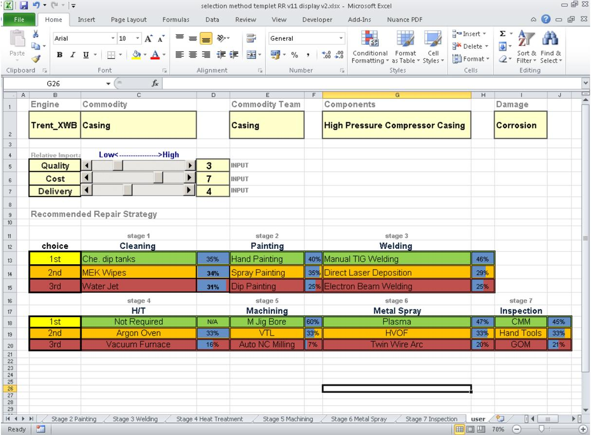
Figure 81 ORSS output for validation of case 1
