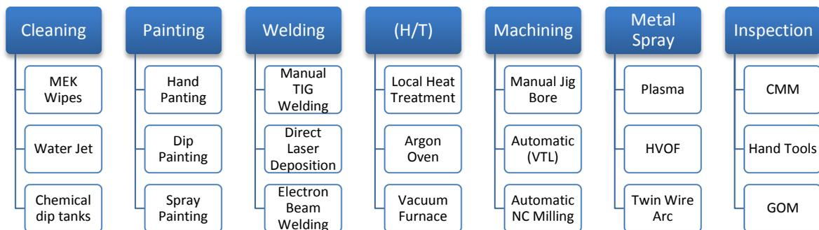
Figure 52 Components Repair process activities
