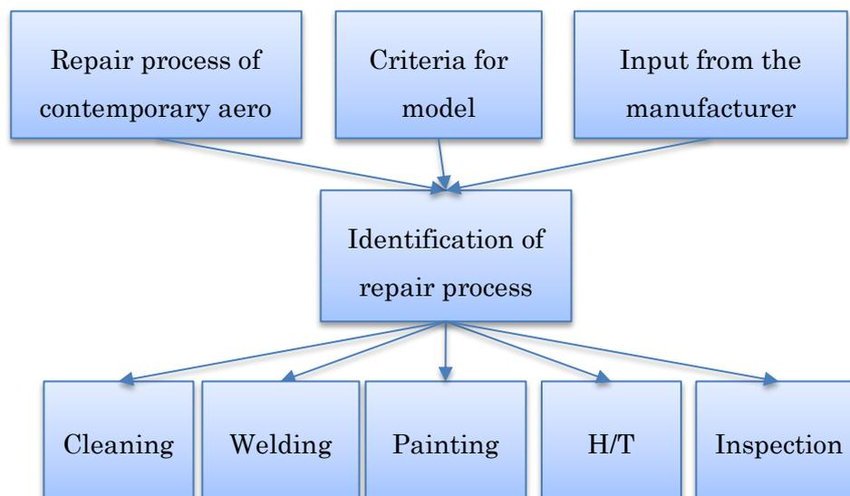
Figure 51 Development of repair scheme
