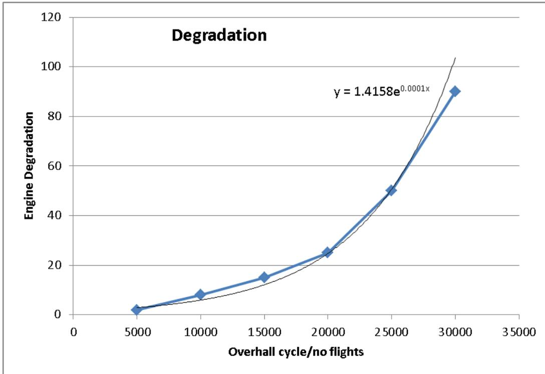
Figure 63: NGV Performance Degradation
