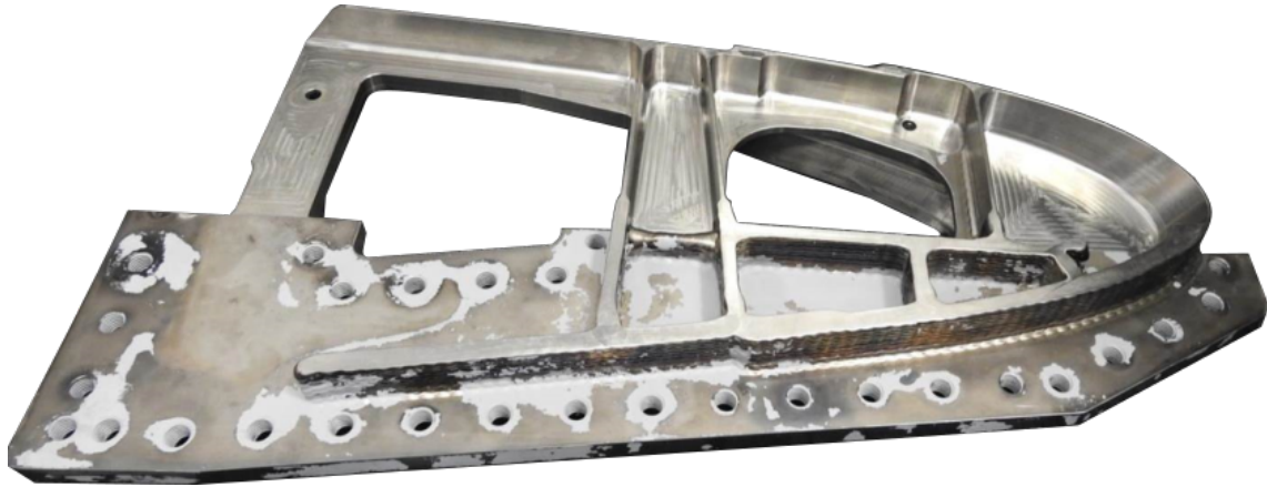
Figure 1.1: Half machined part built using the WAAM technology
