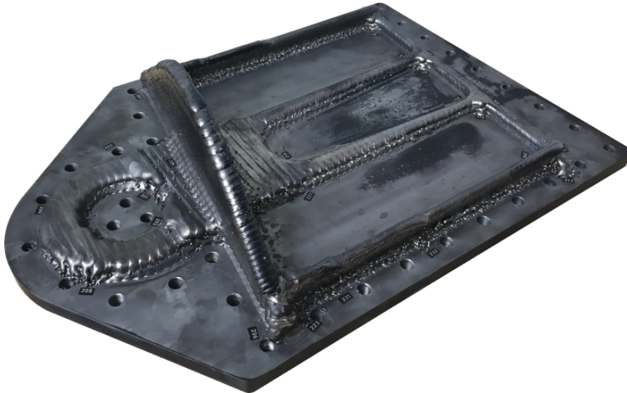
(b) Final part; the dark color is a result of the heat treatment
