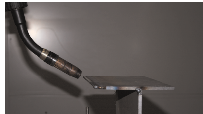
Figure 2.16: Horizontal wall building with torch angle [28].
