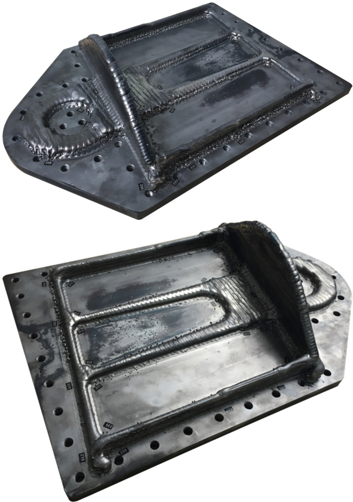
Figure A.7: Resulting pylon component after heat treatment
