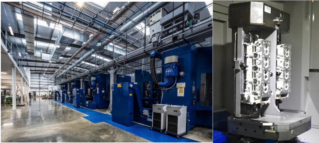
Figure 25 FMS Shop floor (left) and engine part installed on pallet (right) from selected case study (from Cosworth)
