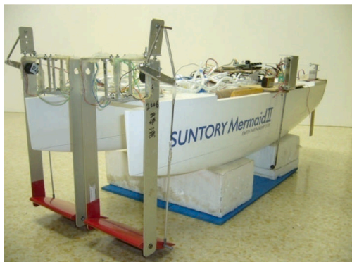
Fig. 14. Test model of Suntory Mermaid II equipped with all sensors and WDPs (Terao [80]).
