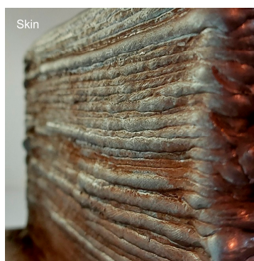
Figure 12. Side view of the demonstrator showing the lower surface roughness of the skin.
