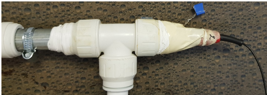
Figure 3-5 Part of the flow loop with LPR probes
