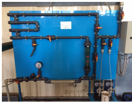
Experiments in flowing water in plastic pipes
