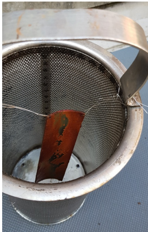
Figure 5-6 B57 Coupon after corrosion before being removed from the bucket
