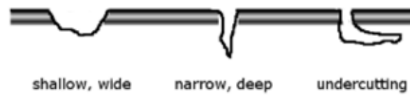
Figure 2-3 Some form of pitting on a metal surface[Nanan 2019]
