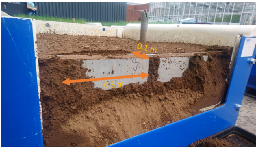
Figure 3-2 Sub-samples using stainless-steel inserts for the bare soil treatment.
