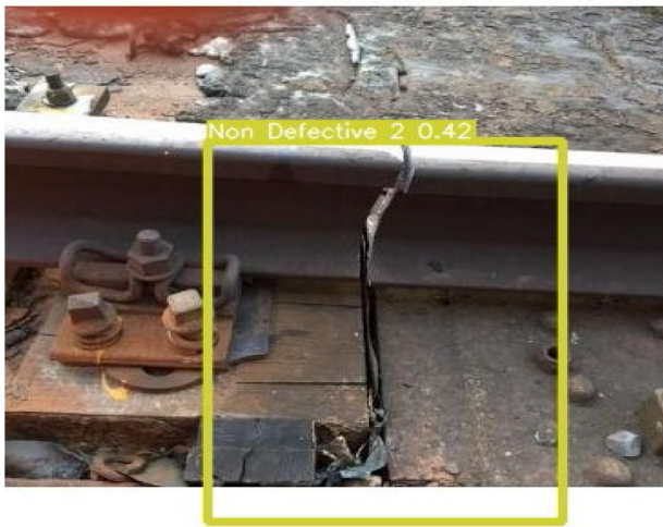
Fig. 14. Defective 2 wrongly classified as non-defective 2.
