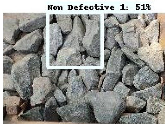
Fig. 19. Non-defective false positive.
