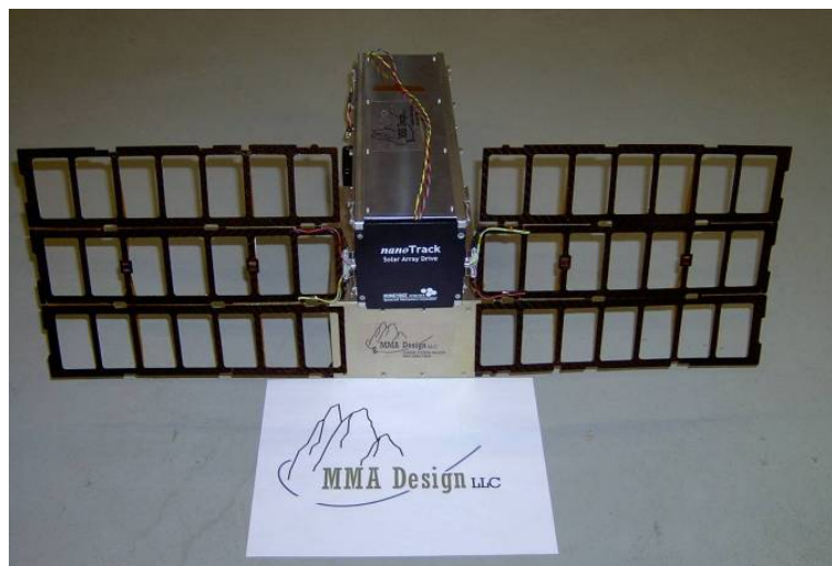
Figure 5-7: HaWK Solar Panel placed on 3U CubeSat with gimbal mechanism [90]
