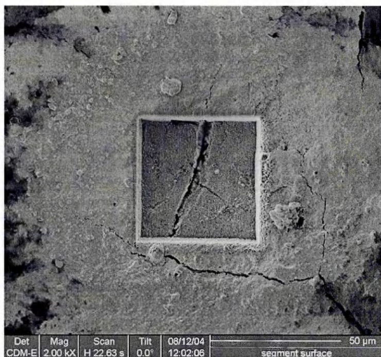
Figure 2.11: Cupwheel segment surface, trough etched with a gallium ion beam on the FIB facility
