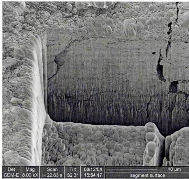
Figure 3.6: Detail of the wall at the left side of the etched area
