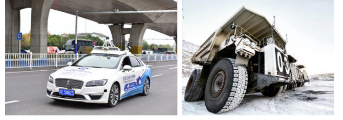
Fig. 4. The figure shows the appearance of IVs. The left vehicle is the test autonomous platform of Xi'an Jiaotong University. The right vehicle is the autonomous mining truck at an open-pit mine in China.
