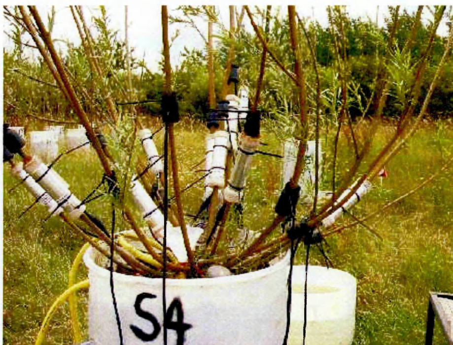
Figure 4.4 Dynagages installed on ten stems of the coppiced willow plant, grown in a lysimeter. Also shown is the 110 mm funnel positioned to collect throughfall precipitation and the foam collars and a length of plastic tubing attached to each stem to deflect stemflow water out of the lysimeter.
