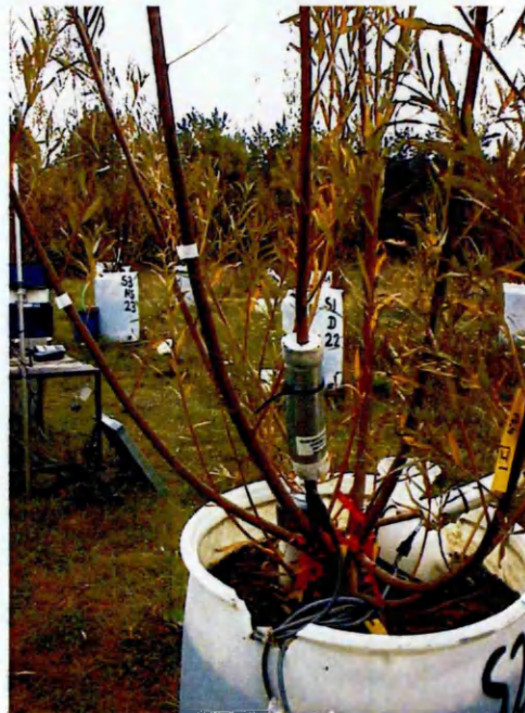
Figure 3.1 Lysimeter with coppice willow plant and Stem heat balance sap flow gauges installed on two stems (2001 experiment).
