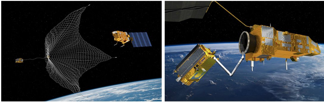
Figure 1.2: Computer-generated renders of potential active debris removal (ADR) approaches developed for the European Space Agency’s (ESA) e.Deorbit mission. (Left) Capture with net attached to tether. (Right) Capture with robotic arm.
