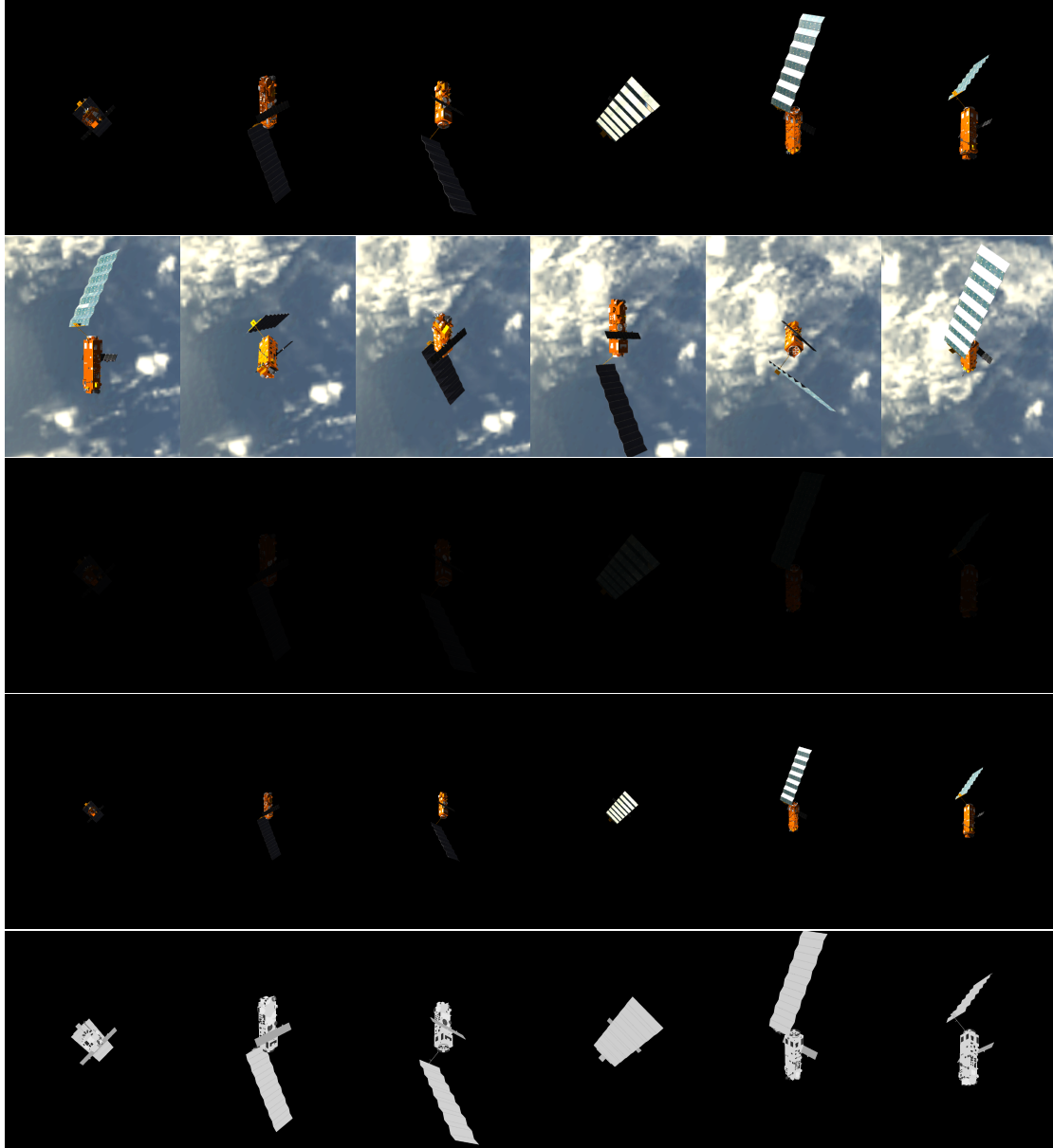
Figure 2.15: Characteristics of the ASTOS dataset. ( Top Row ) A continuous sequence of red-green-blue (RGB) images in the visible wavelength of the target Envisat as imaged by a chaser's on-board camera. ( Second Row ) Earth contaminating the background. ( Middle Row ) Imaging during eclipse periods. ( Fourth Row ) Relative proximity changes. ( Bottom Row ) Imaging in long-wavelength infrared (LWIR).
