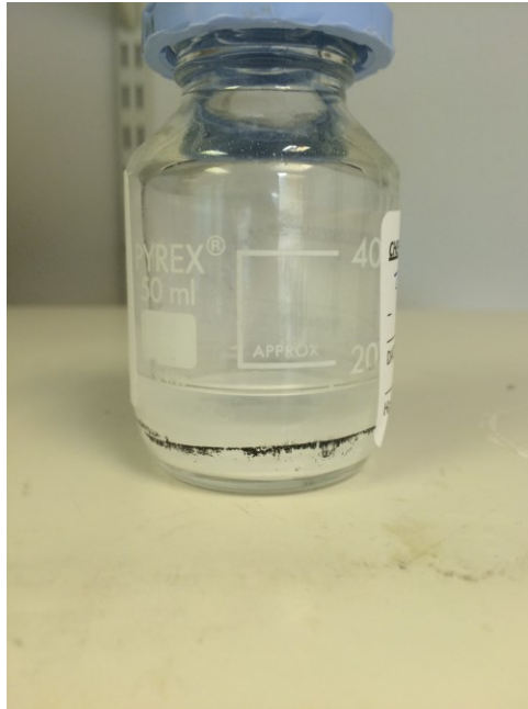
Figure A 4 sample showing the sedimentation of YSZ
