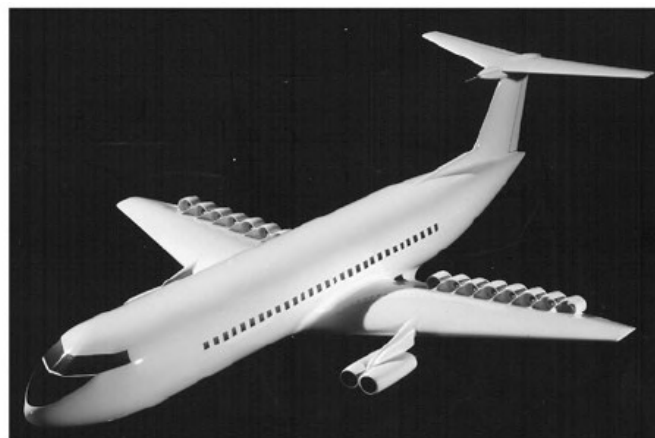
Figure 3: Early distributed propulsion concept
