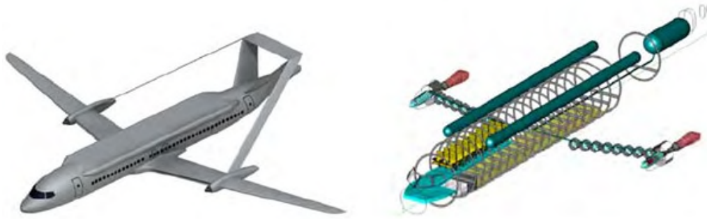
Figure 4: NASA advanced cryogenic electric propulsion system
