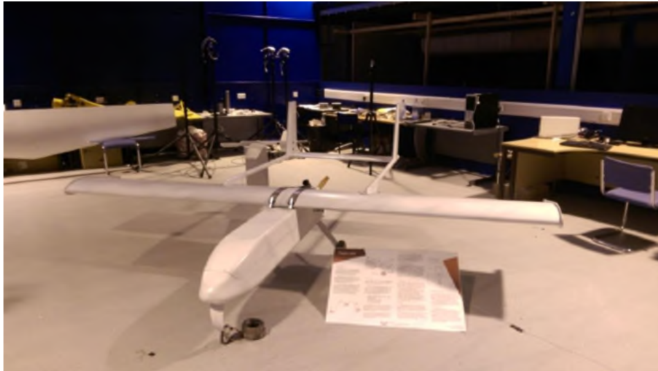
Figure 5-1: Photograph of model Aegis UAV with U-tail configuration at Cranfield University, the A1 sheet of paper gives an indication of model size
