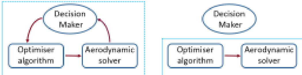
Figure 3-2: Left panel; the preference base design loop (interactive). Right panel the conventional design loop (non-interactive)
