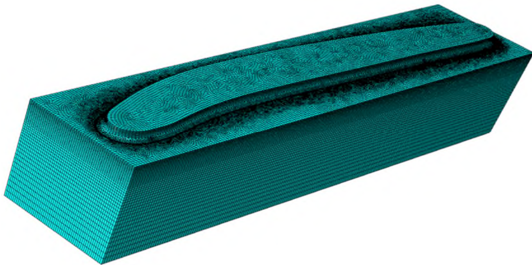
Figure 6-3: Blisk like mesh
