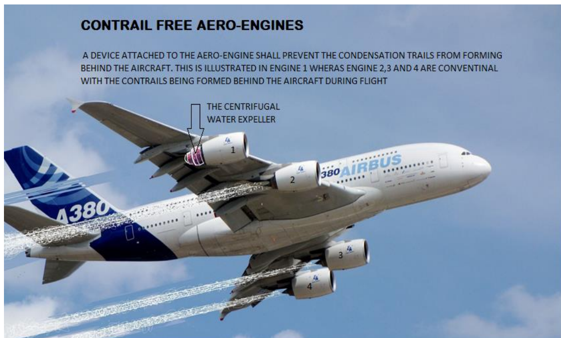
Figure 1-2 : The Centrifugal Water Expeller Integrated into the Core Engine (Courtesy: Airbus for A380 Photograph)
