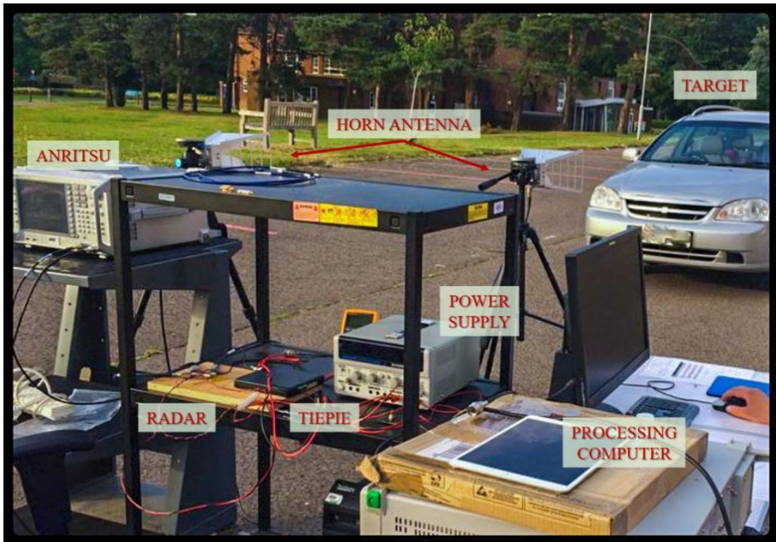
Figure 5.16: A 3.5 GHz FMCW Radar Experiment Arrangements
