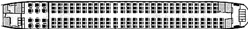
Figure A.34 Boeing 737-900 interior arrangement, 177 passengers (mixed class), first class at 36-in pitch, economy class at 32-/31-in pitch (Ref. 2.38)
