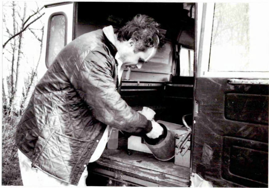
Plate 4.4 Assembly and lubrication of the sampling cylinder.
