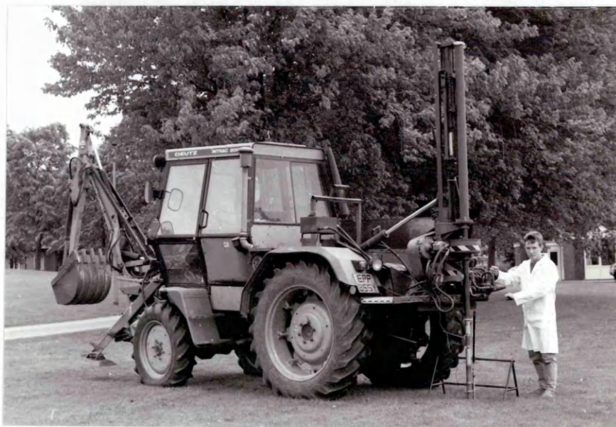
Plate 4.3 The Deutz Intrac tractor adapted to accommodate soil assessment equipment.
