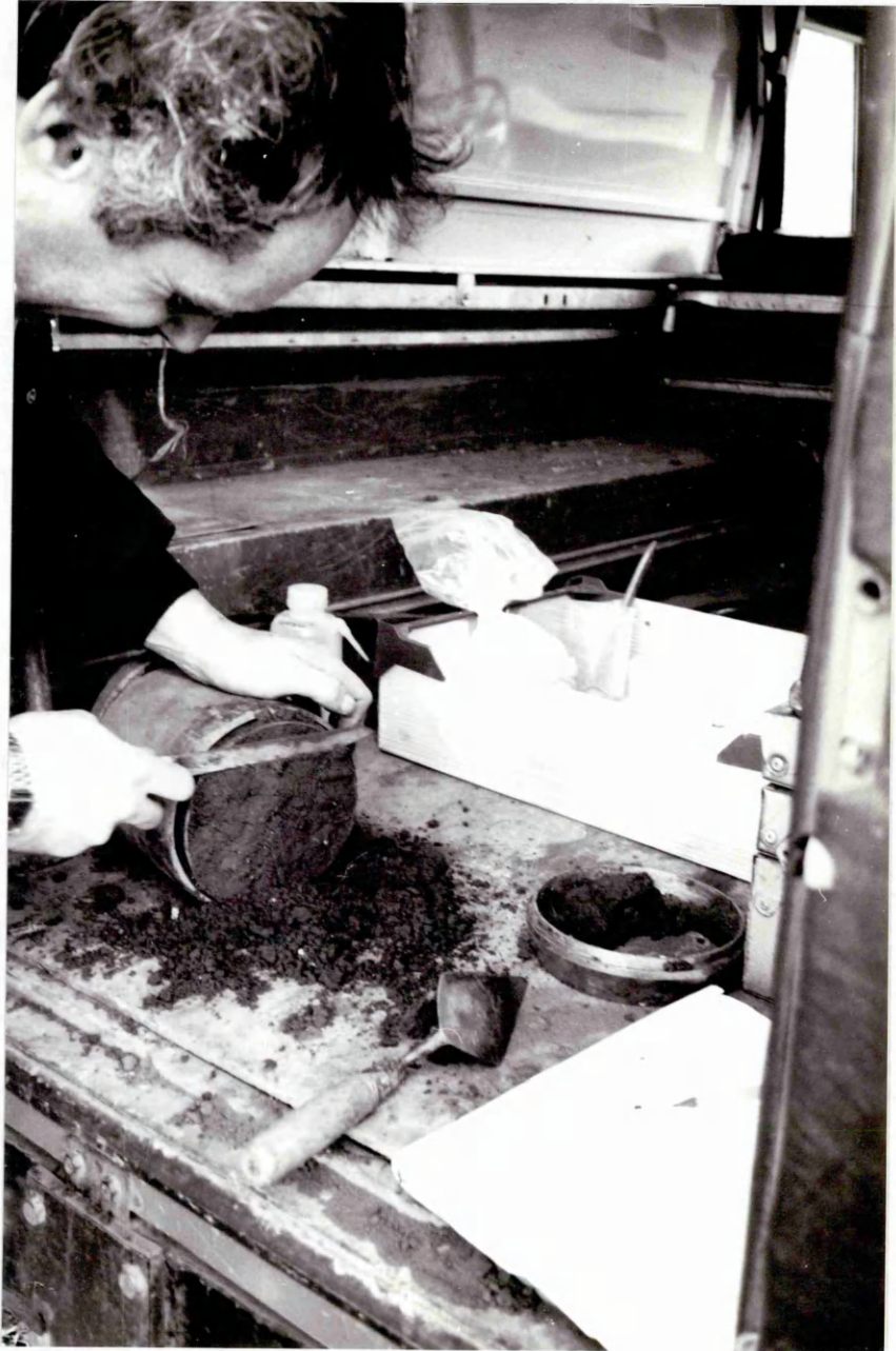
Plate 4.7 Trimming the ends of the soil sample within the confining cylinder.
