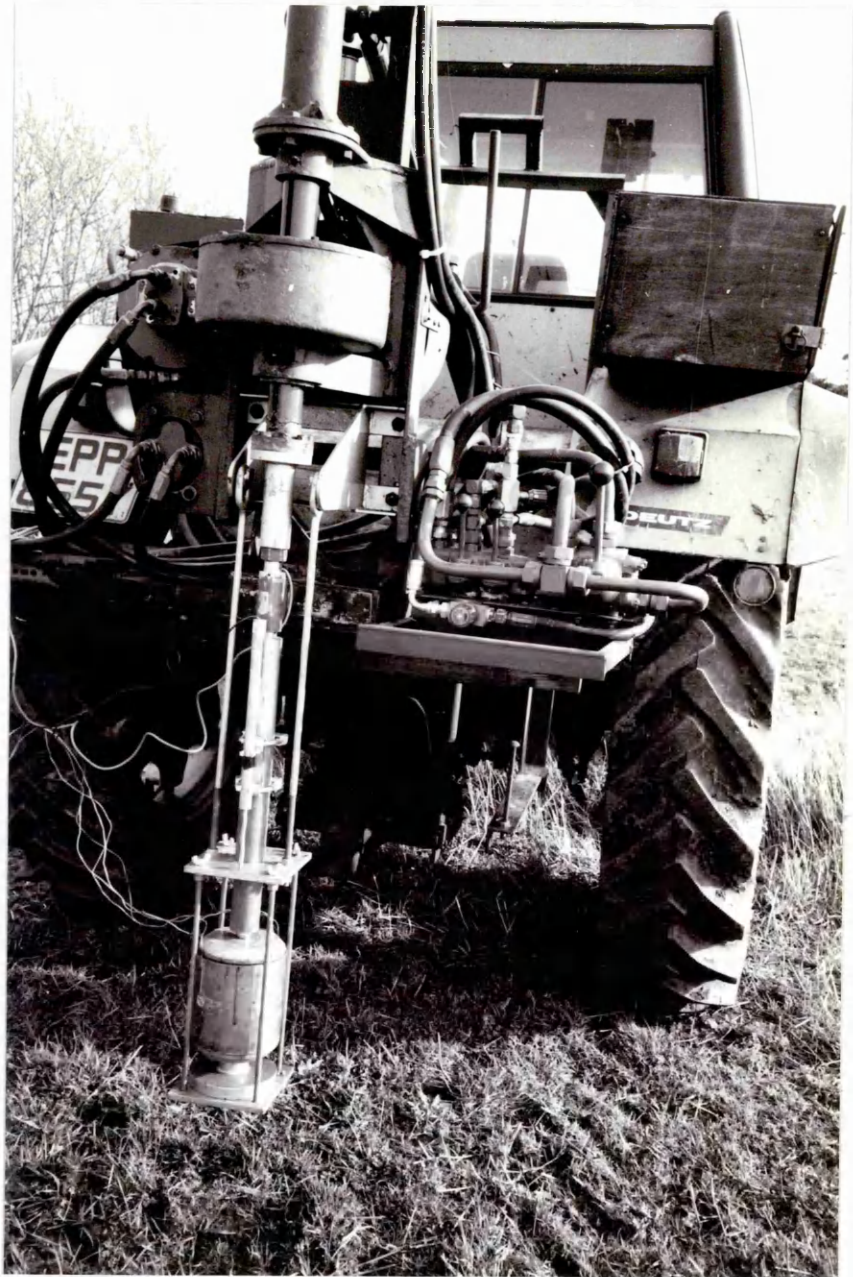
Plate 4.8 A confined compression test.
