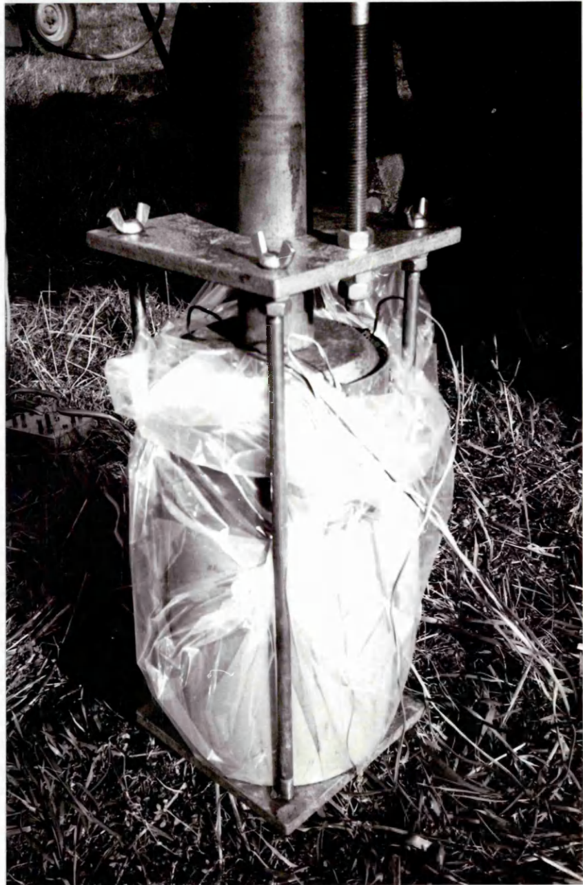
Plate 4.9 Extruding the soil sample.
